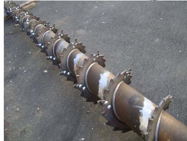
***New design with ceramic layer to ensure long life time (2 years)***
